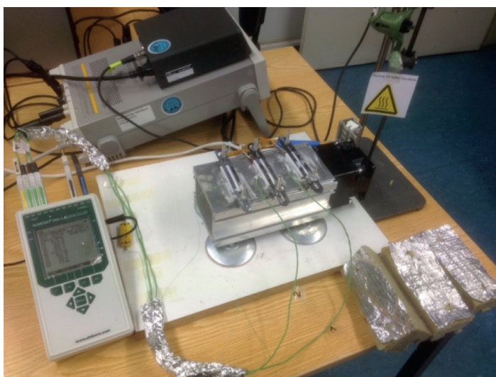
Picture 7: Three heaters a 175 W (525W total) mounted on three aluminum plates (55mm x 20mm x 2mm) with heat transfer paste Alutronic PA700 and 2mm Teflon isolation.
